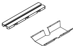
**Double cable duct\* hinged in both sides**
