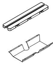
**Double cable duct\* hinged in both sides**
